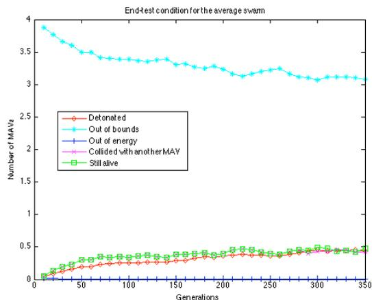
Fig. 8. End-test condition for the members of the "average" swarm. The plot shows, during a typical test, how many MAVs detonate, exit from the environment boundaries, run out of energy, collide against a team-member, or survive
