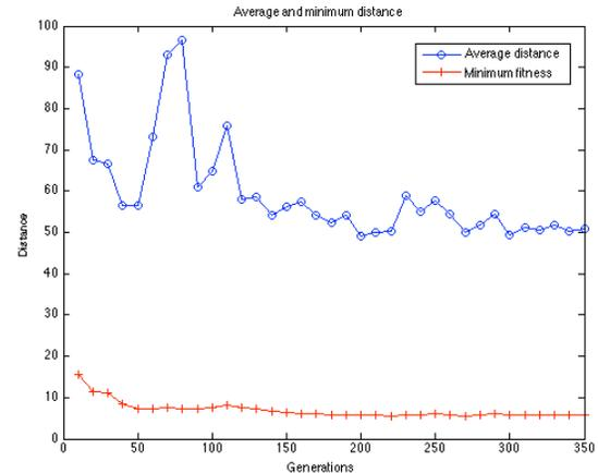
Fig. 5. Average and minimum distance between the target and the detonation point of the MAVs detonated closest to it
