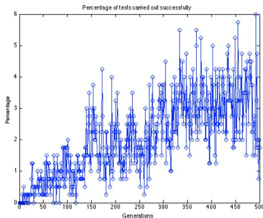
Fig. 10. Percentage of tests concluded successfully for a MAV team made of a single member. As it is possible to see into the plot, the success rate merely reaches a maximum of 6% in 500 generations
