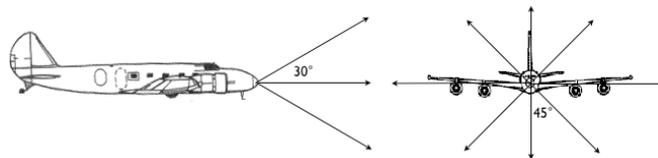
Fig. 9. Isometric side and front views that show how the ultra-sonic sensors could be deployed on the MAVs
