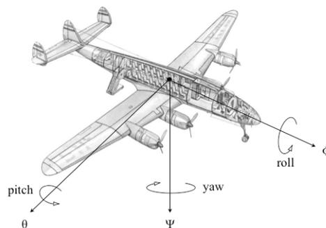
Fig. 2. The degrees of freedom available to a typical fixed-wing aircraft
