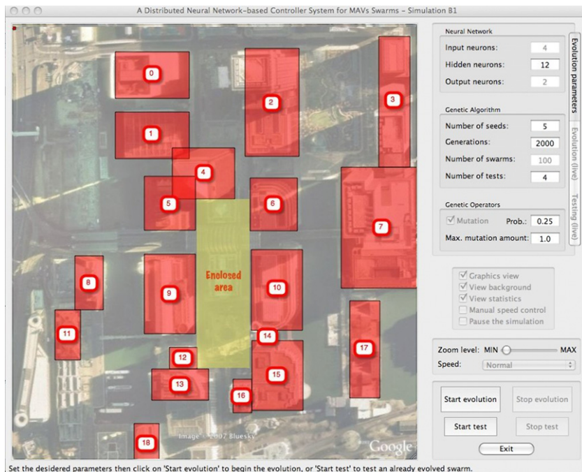
Fig. 1. A screenshot of the 2D simulator. On the left it is possible to see the environment used in this model. The obstacles, corresponding to the tallest buildings present in the Canary Wharf area, have been highlighted.
