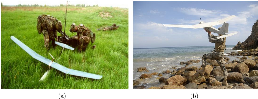
Figure A.3: (a) AV Pointer FQM-151A; (b) AV Puma AE (All Environment). Sources: (a) <http://www.avinc.com/uas/adc/pointer/>; (b) [http://www.avinc.com/uas/small\\_uas/puma/](http://www.avinc.com/uas/small_uas/puma/)
