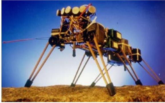
Figure 2.3: Genghis the robot. One of the first robots built by Rodney Brooks' research group relying on the Behaviour-based robotics approach. Source: <http://www.ai.mit.edu/projects/genghis/>
