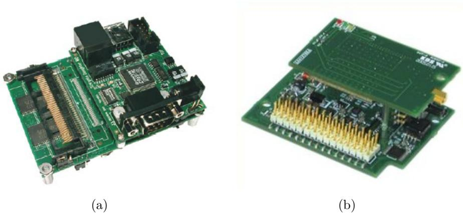
Figure B.1: (a) Crossbow SPB400 Stargate Gateway; (b) Crossbow MNAV 100CA Inertial Measurement Unit. Sources: (a) [http://www.willow.co.uk/html/spb400-stargate\\_gateway.html](http://www.willow.co.uk/html/spb400-stargate_gateway.html); (b) [http://www.gpsarea.com/p\\_detail.asp?ID=412](http://www.gpsarea.com/p_detail.asp?ID=412)
