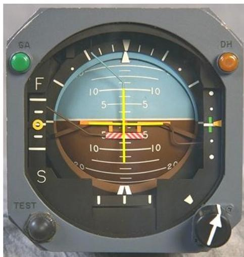
Figure 3.9: An Artificial Horizon (AH) device. Source: [http://en.wikipedia.org/wiki/Attitude\\_indicator](http://en.wikipedia.org/wiki/Attitude_indicator)
